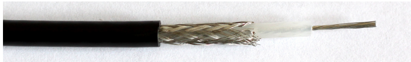
↑ Pastic jacket (PVC) ↑ Outer conductor 'Shield' (aluminium) ↑ Insulator (PE) ↑ Inner conductor 'Core' (copper)
